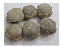
ARM 72 is an agglomerate of reactive magnesia, available in the form of briquettes or lumps that can be used by the steel industry's demand enhancing refractory performances.
