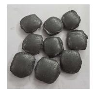
ARM 72 is an agglomerate of reactive magnesia, available in the form of briquettes or lumps that can be used by the steel industry's demand enhancing refractory performances.
