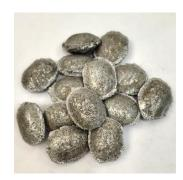
BASS is a bailed briquetted aluminium shredded scrap, available in the form of half cones, briquettes or ingots that can be used by the steel & foundry industry's demand for aluminium-killed steel.
