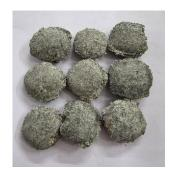
**FLAMBAS-35** is a mild fluoride with lime, alumina, magnesia, briquetted with aluminium shredded scrap, available in the form of half cones, briquettes, or ingots that can be used by the steel & foundry industry.
